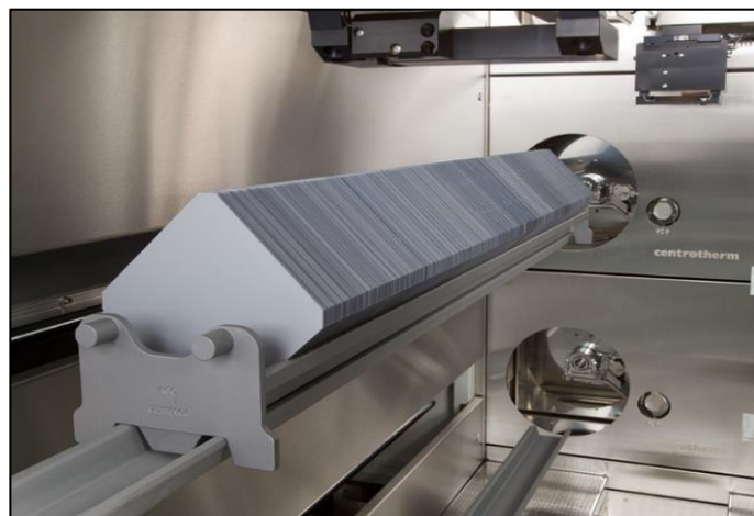
High-capacity diffusion boot with back-to-back loaded wafers
