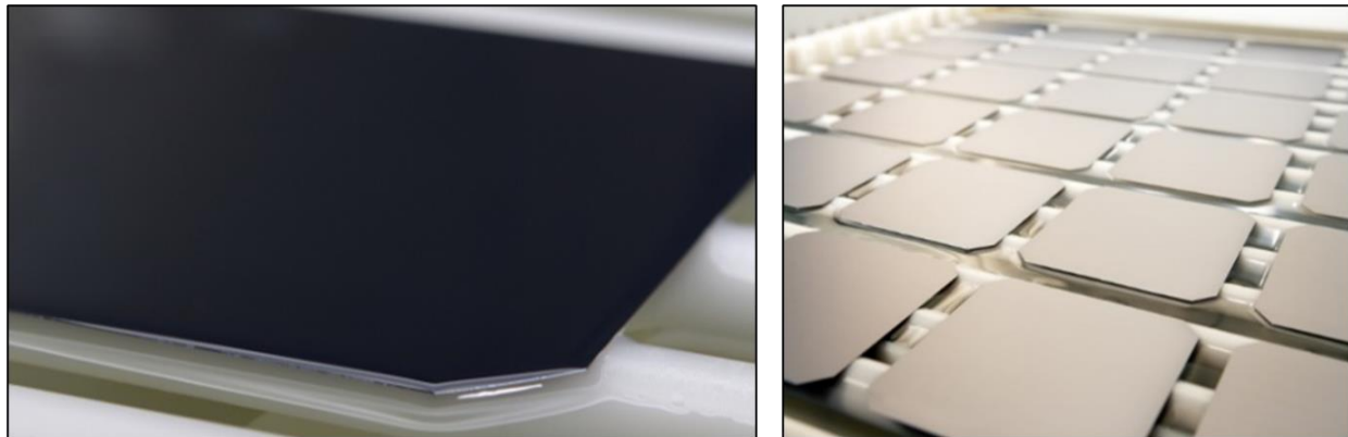
Fig 2.6 Rear Side Etching for Edge Isolation in main Etching Bath of 5-lane Industrial Inline
